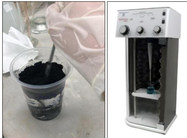
Figure 3. Process of Mixing CNF Using the Ultrasonic Apparatus
